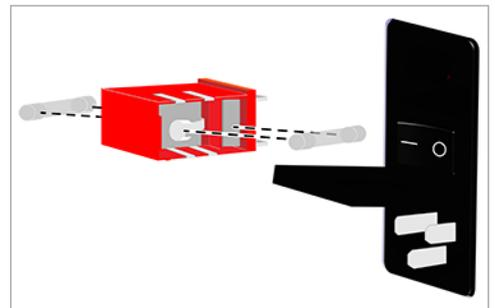
5. Insert the fuse cartridge into the power inlet housing.
