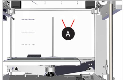
14. Mount the jet wiper mounting posts to the back panel of the printer through the keyhole slots.
