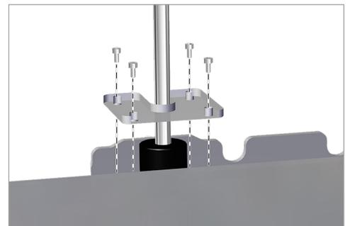
12. Using a 4mm hex head driver, attach the mounting posts to the jet wiper assembly with the supplied screws and washers.
