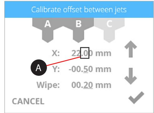
11. Press the up arrow three times to increase the value to 22.30 mm.
