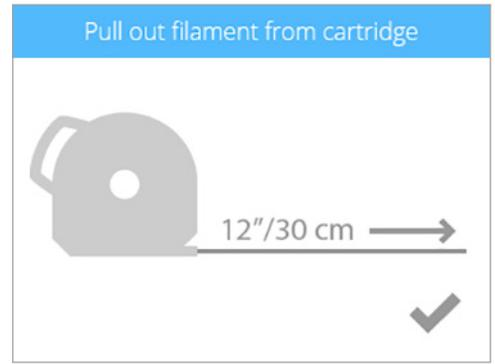
5. Cut off 2"/5 cm of material from the end. Select the **checkmark** to continue.
