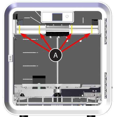
11. Loosen and remove the four (4) 4mm screws securing the Z-Axis guard and remove the guard. Save the guard and screws for future repacking.
