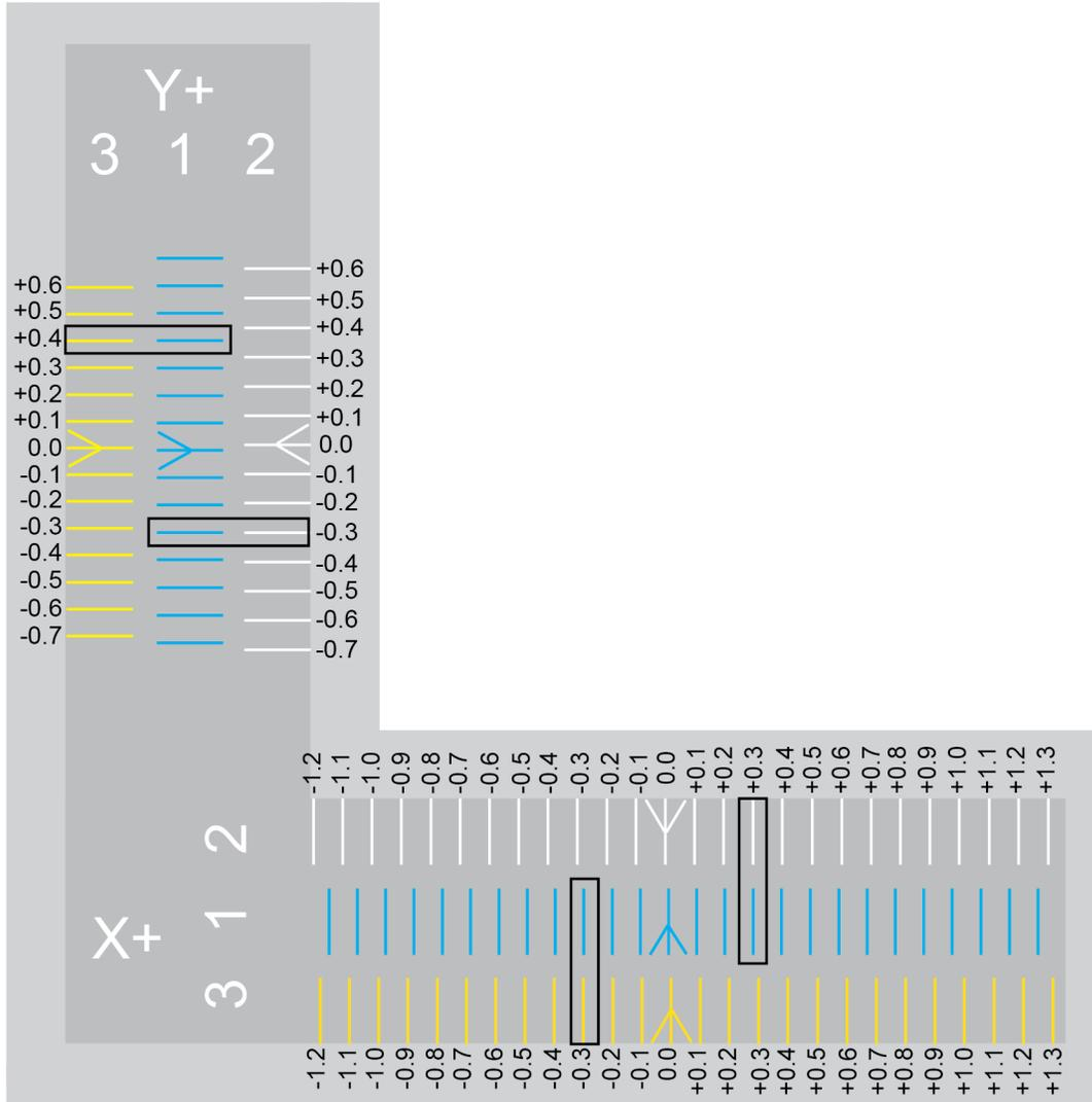
Note the white arrow printed from print jet 2 and compare it to the positioning of the blue arrow printed by print jet 1. Note that the white arrow is slightly left of the blue arrow meaning that print jet 2 is misaligned. Print jet 2 must be moved in a positive direction (right) to align with print jet 1.
