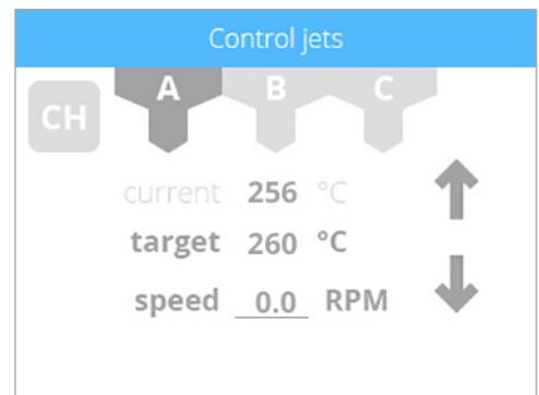
5. Once you have finished, reduce the target speed to 0.0 RPM and the target temperature to 0.0°C. You can now select the next print jet and follow this procedure if necessary.
