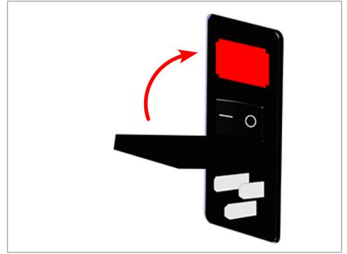
7. Connect the printer power cord and power on the printer.
