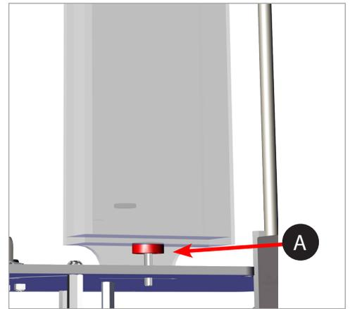
7. If the wiper tip is too low, remove the jet wiper assembly and turn the adjustment thumbscrew (A) counter-clockwise. Reinstall the jet wiper and return to step 5.
