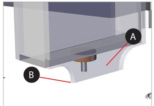
16. Remove the print pad from the box and place it onto the print platform with the round magnet on the bottom of the pad inserted into the triangular opening on the platform. Ensure the print pad is securely seated on the print plate.
