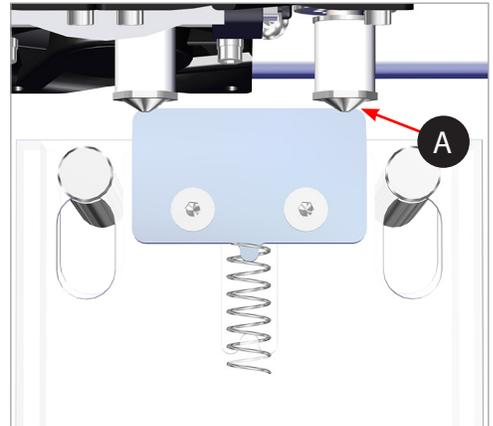
6. If the wiper blade is too high, remove the jet wiper assembly and turn the adjustment thumbscrew (A) clockwise. Reinstall the jet wiper and return to step 5.
