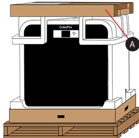
5. Remove the upper foam supports (A) from the printer.
