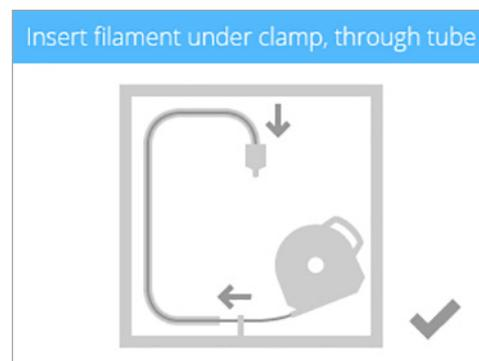
16. Continue to manually feed the print material through the material tube until it begins to extrude from print jet 1 into the jet wiper assembly. Select the **checkmark** to continue.
