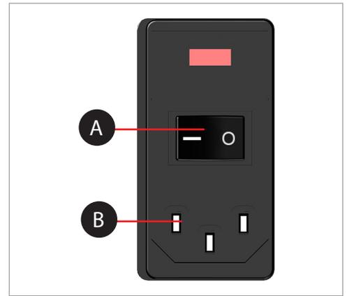
18. Press the on/off button (A) beside the LED screen to power on the CubePro touchscreen display.
