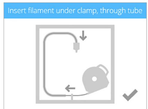
11. Gently push the material into the print jet until molten plastic extrudes into the jet wiper. Select the **checkmark** to continue.
