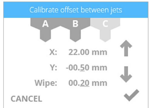
10. Referring to the illustration at the beginning of this procedure, print jet 2 needs to be increased by .3 mm. Select the value until the first digit (A) to the right of the decimal point is highlighted.
