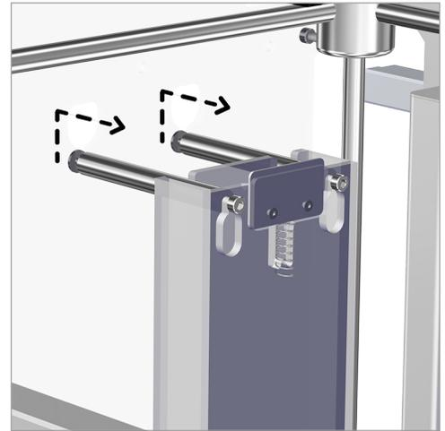
3. Remove the jet wiper assembly from the printer.
