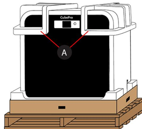
6. Pull the protective bag down around the printer and remove the printer assembly from the lower foam support.
