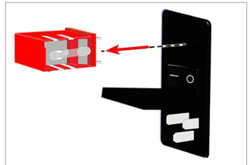
4. Remove the defective fuses and install new ones.
