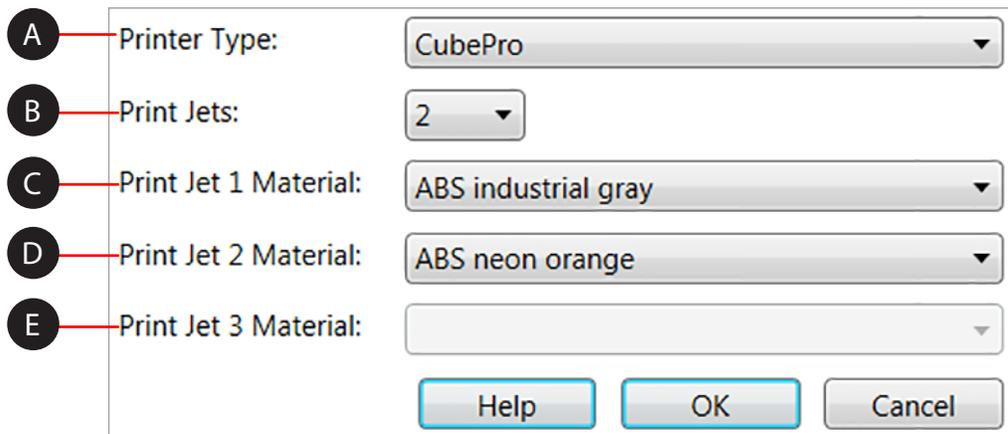
The image shows a 'Printer Configuration' dialog box with five rows of settings, each labeled with a letter in a circle (A-E) and connected to the setting by a red line. The settings are: 'Printer Type' set to 'CubePro', 'Print Jets' set to '2', 'Print Jet 1 Material' set to 'ABS industrial gray', 'Print Jet 2 Material' set to 'ABS neon orange', and 'Print Jet 3 Material' which is currently empty. At the bottom of the dialog are three buttons: 'Help', 'OK', and 'Cancel'.
